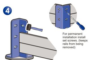
Assemble all (8) bottom rails first. Next assemble the second row and last the third row. Secure and interlock vinyl rails by tapping with rubber mallet.
