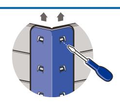
**DISASSEMBLY:** Insert large slot screwdriver into the tab opening as shown. Push up on screwdriver and the vinyl rail will lift. Remove rail by hand.
