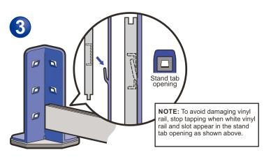
Starting with the lowest rail and with the tongue down and groove up, align the rail opening with the stand tab. Push into place. Tap with a rubber mallet to secure vinyl rail to stand.
